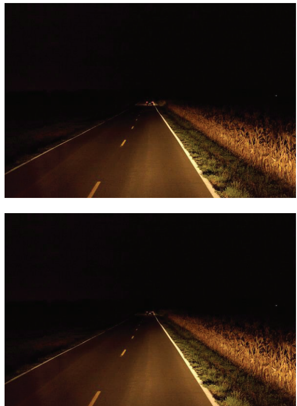
Figure 2. Bright Taillights (top) and Dim Taillights (bottom) from same distance of 128 m.
